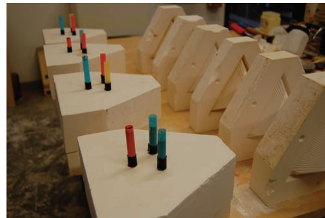
44. Slip casting production line
