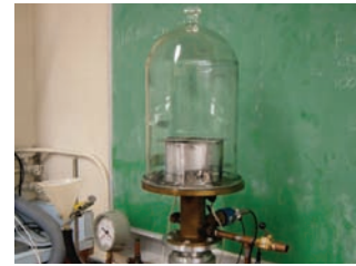
22. vacuum chamber for aluminizing resin samples
