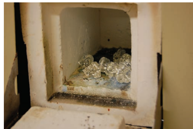
18. Glass placed in oven for annealing
