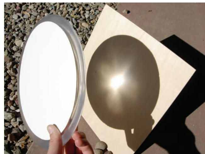
4. Fresnel lens behavior of prism torus.
