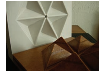
31. plaster cast pulled from form
