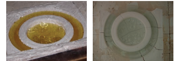
9. Molten glass during annealing process.
