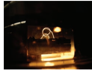
23. heating filament with melted aluminum globules during aluminization
