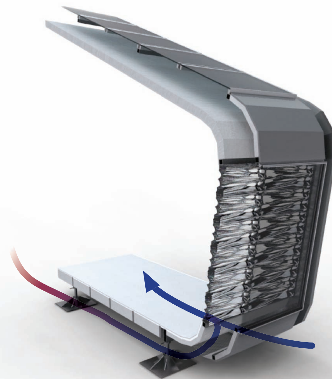
Summer Night Time Air can be brought in from below the home and through the south wall to provide natural ventilation to the interior space.
