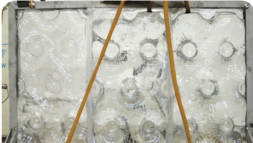
Panel system using vacuum pump and hydraulic connection lines. Exploration in filling and evacuation strategies.
