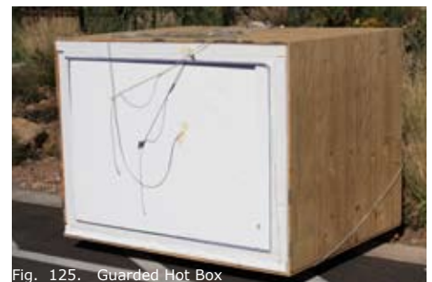
Fig. 125. Guarded Hot Box
