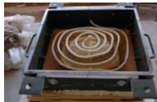
Fig. 95. Mold ready to cast
