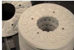
Fig. 81. Slip casting molds
