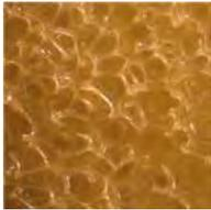
Fig. 1.1 polyurethane foam
