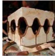
Fig. 7.7 slip cast plaster mold
