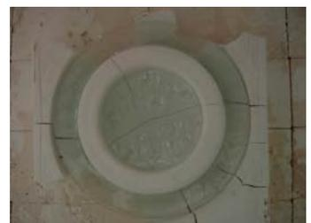
14. The waste mold is pulled away from the glass.
