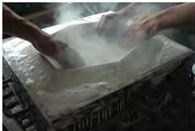
Pressurizing the plaster production mold
