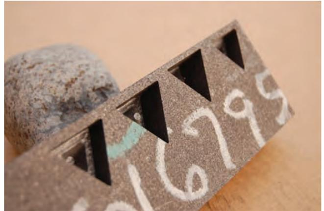
8. Machined graphite mold block
