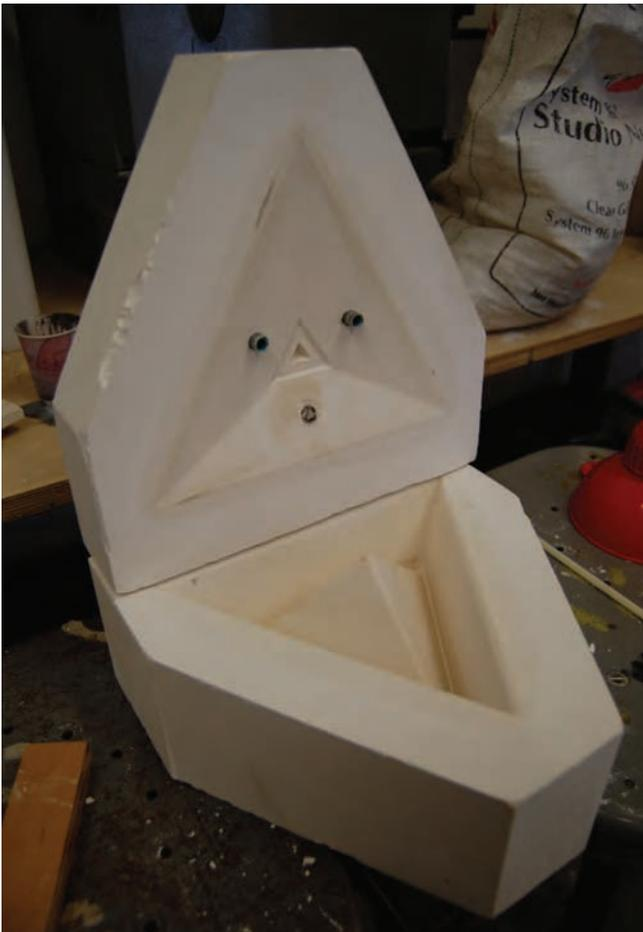
45. Pottery plaster molds for slip casting
