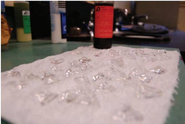
22. Final polish with 9 micrometer polycrystalline diamond lubricant
