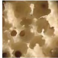
Fig. 1.2 fired ceramic from polyurethane foam
