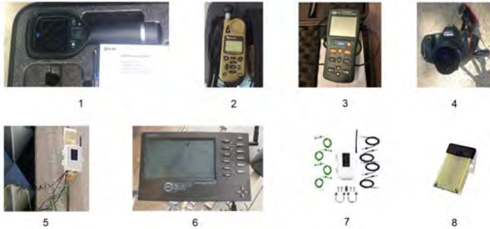
Figure 5: Equipment for measurement campaign for 2019 and 2020. 1-FLIR E6 thermal imaging camera, 2- Kestrel 2400 Heat Stress Tracker, 3 – Solar Meter, 4- Canon EOS fisheye camera, 5- Davis weather station, 6- Davis Vantage Pro 2, 7 – soil moisture and temperature probes, 8 – leaf temperature and wetness sensor. Source: (Authors 2021)
