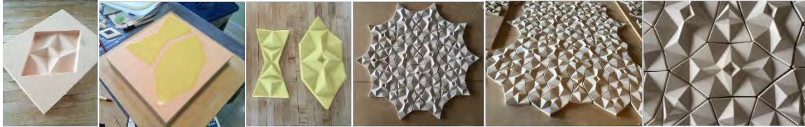
Figure 10: Slip casting process of the quasi-periodic units. Source: (Ajlouni 2021)
