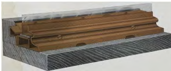
Figure 2 “Metal Sash No. 30.” One of Kawneer’s first products was a copper clamping system that formed a sash around storefront windows. Source: Kawneer Store Fronts, 1912.
