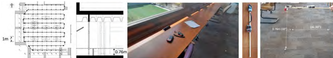
Figure 3: From left to right: Floor plan showing grid of measurement locations; partial sectional drawing showing height of measurements at the work surface level; light-meter tool used to measure illuminance; light meter with extension rod for sensor; light meter with extension rod held 30 inches above the floor finish. Source: authors.
