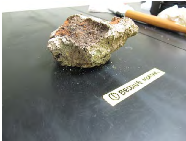
Figure 15: Photo of bulk bedding mortar sample.
