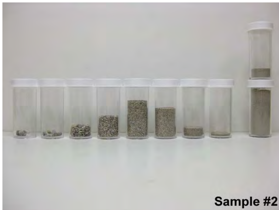
Figure 3: Photographs of the sand extracted from the two samples by acid digestion after gradation through a standard sieve stack. Particle size distributions are broad for both though the sand in Sample #1 is coarser-grained. The vials set aside to the right in each image represent fines passing a No. 325 sieve. Though some of this may represent undigested silica from the binder, much of it is volcanic rock fragments and glass. This may simply represent unwashed clay-sized fines from the sand source. Alternatively, these may represent a separate natural trass addition.
