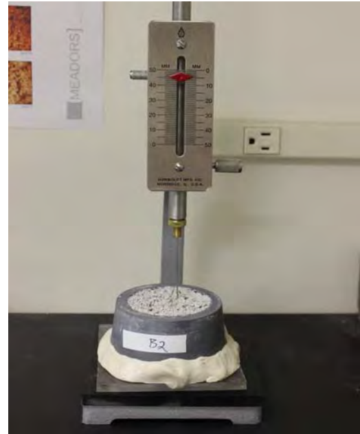
Figure 26: Formulation B undergoing setting time testing.
