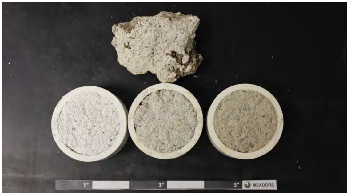
Figure 39: Original mortar (top) with unpigmented replication mortar (left), 1/1024 parts pigmented mortar (middle), and 1/512 parts pigmented mortar (right).
