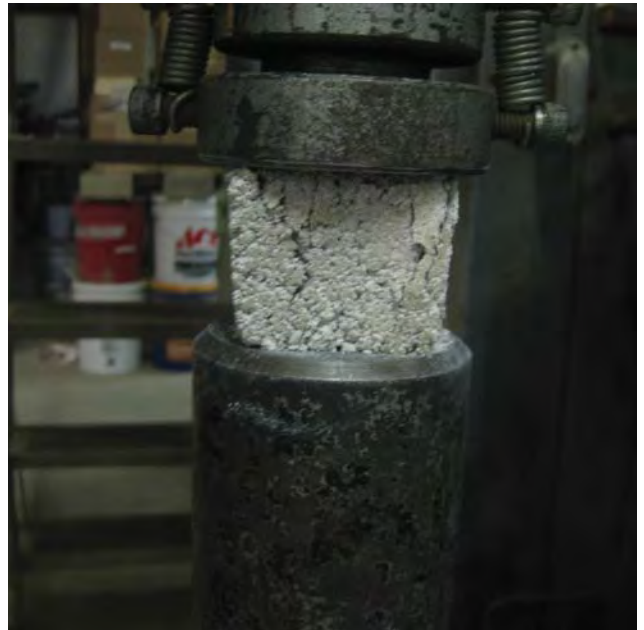
Figure 4: Formulation B undergoing compressive strength testing.
