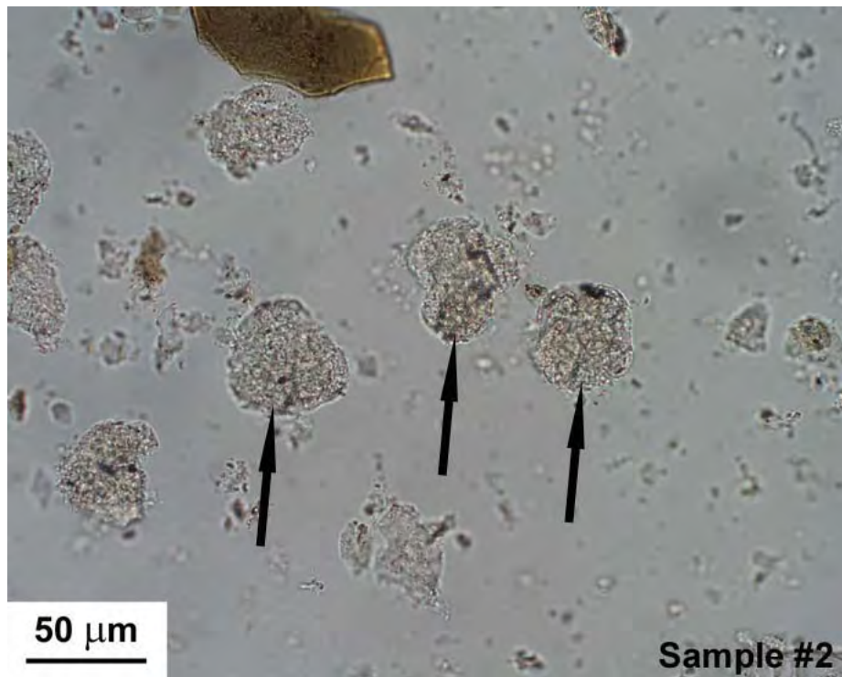
Figure 5: PPL photomicrographs of powder mount specimens prepared from the fines extracted through acid digestion. The arrows indicate fine particles of volcanic glass that represent a major portion of the finest fraction. Refractive indices are approximately 1.50 indicating a high silica content and this would be expected to result in a higher pozzolanic potential.
