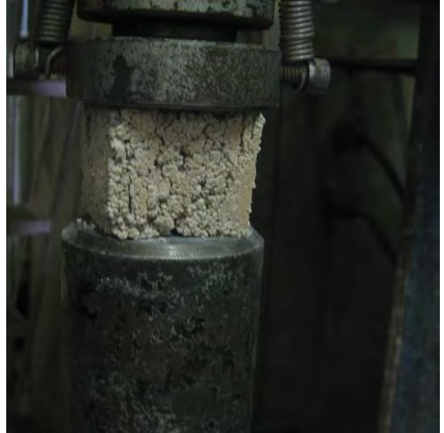
Figure 6: Formulation C undergoing compressive strength testing.
