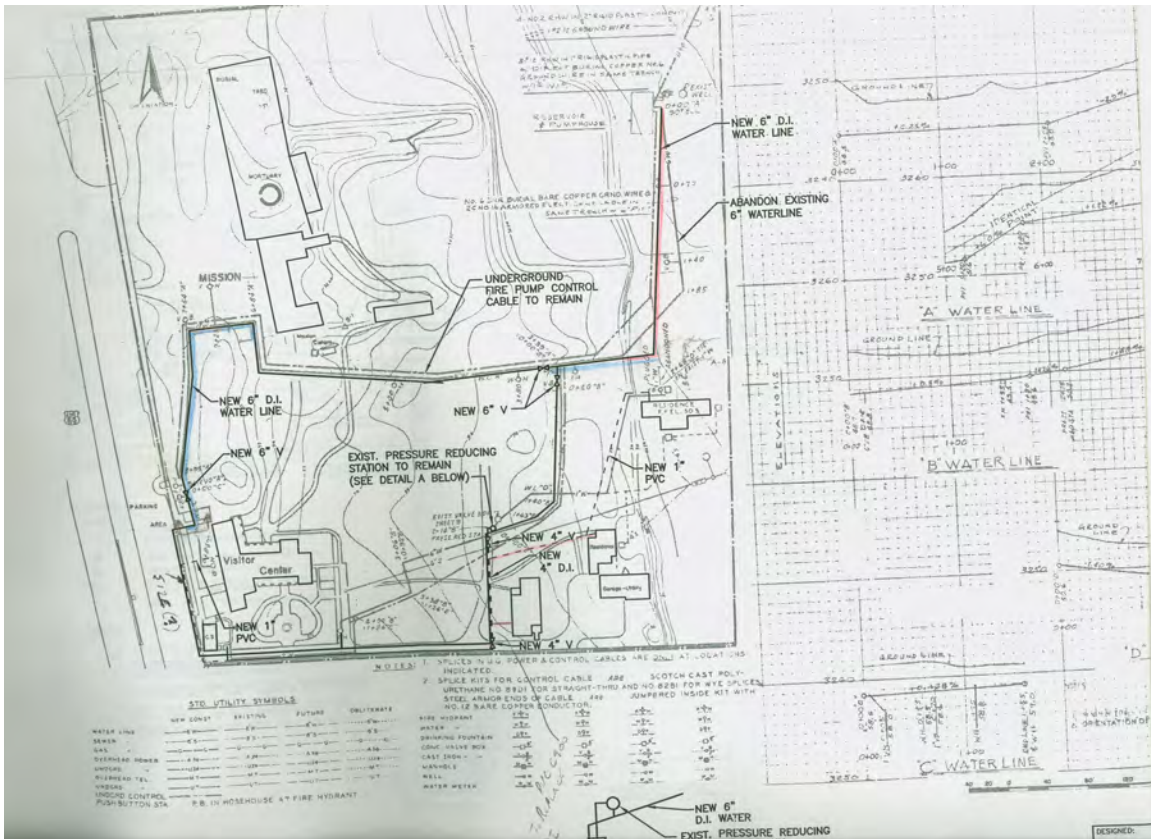
Figure 3.6. Schematic map of Park utility infrastructure produced in 2001. Note existing 6-inch waterline and underground fore pump control cable in vicinity of acequia alignment (NPS TNHP Archives).
