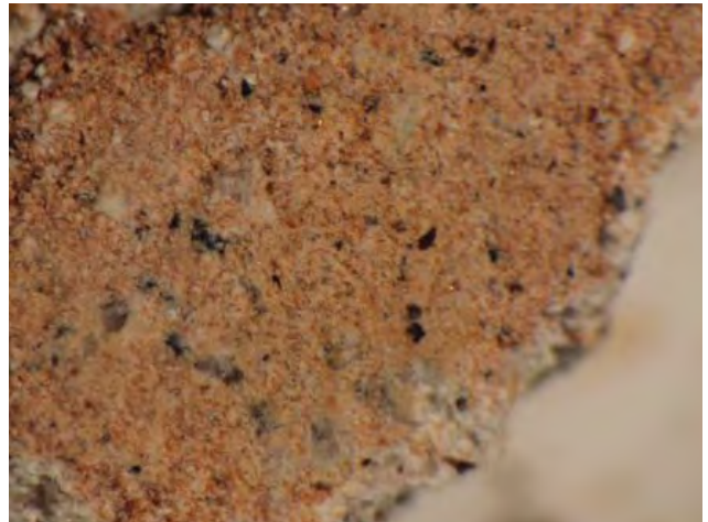
Figure 44: Mexican brick fresco sample. Samples using either brick were identical in color (Munsell color code of 5YR 7/4 “pink”) and texture. Note: Even distribution of brick dust and darker appearance than limewash. (30x magnification, Reflected/Quartz Halogen)
