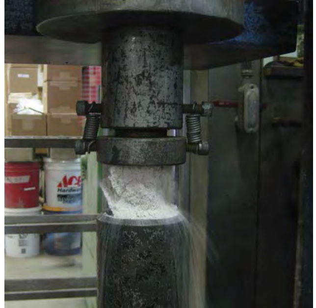
Figure 2: Formulation A undergoing compressive strength testing.
