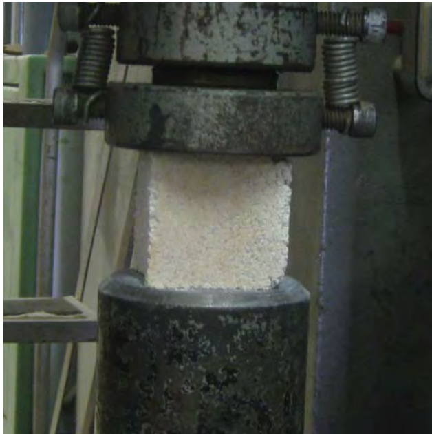
Figures 37 and 38: Sample A undergoing compressive strength testing.
