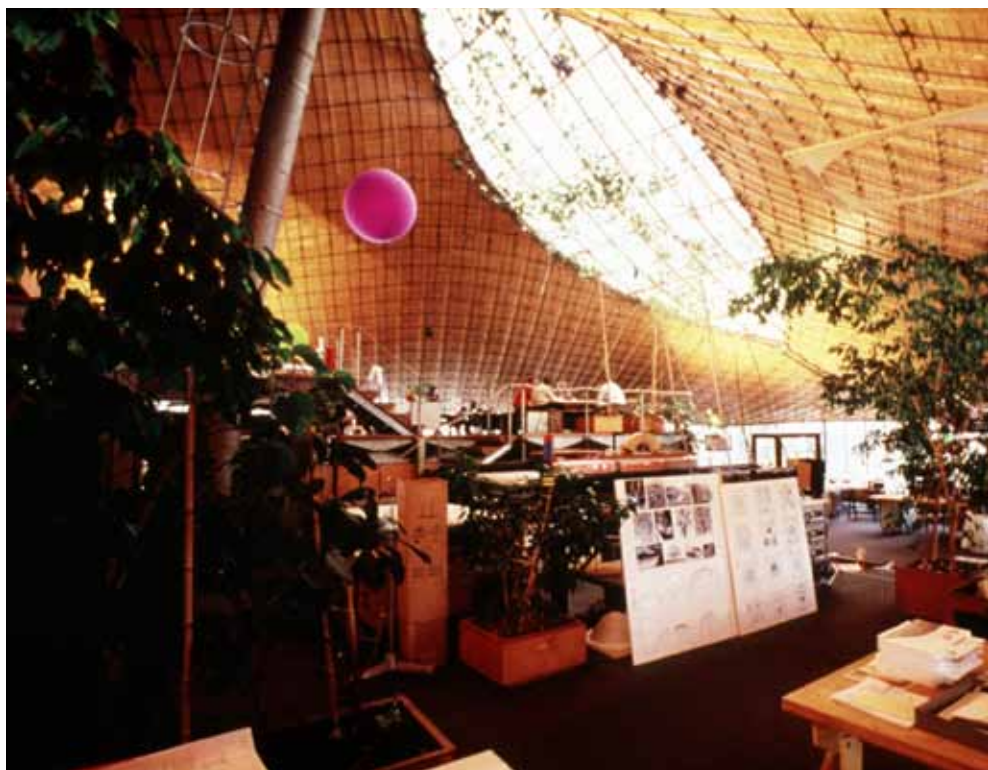
图 2. ILEK Stuttgart permanent structure – interior view of wood ceiling decking attached to steel cable net.
