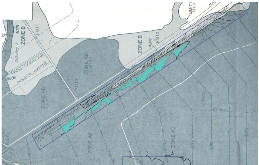
This is a FEMA flood plain map with the site overlaid. The areas shown in light blue indicate areas that would have to be filled with soil in order to be above the flood plain and before being approved for construction.
