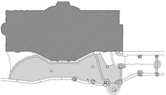
FIG. AT5: Accessibility Alternative Two. In order to create a level surface in front of the Hermit's Rest and provide compliant access through the Great Room entrance, concrete would be poured where hatched, except in the area of the west steps where the concrete steps would be removed.
