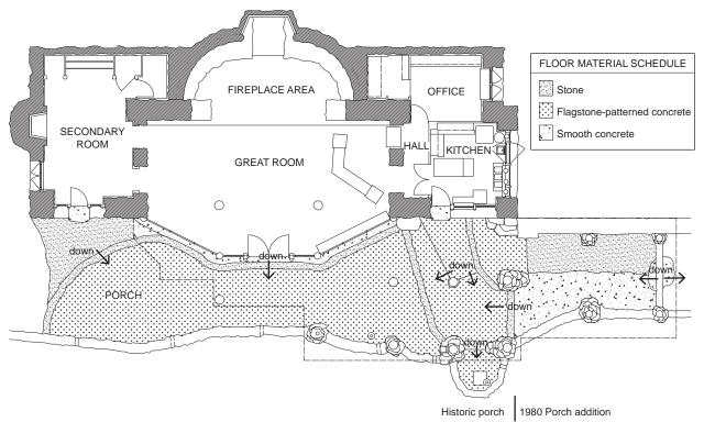
FIG. E1: Plan of the Hermit's Rest showing building perimeter and porch floor, 2007.
