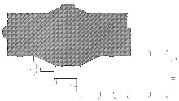
FIG. AT3: Option C for Porch Restoration. The entire roof porch would be reconstructed in the style of the original porch roof with protruding horizontal porch beams.
