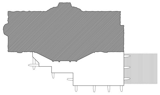
FIG. AT2: Option B for Porch Restoration. The historic porch roof would be restored. The west porch addition would be replaced by a porch roof constructed with compatible materials that are differentiated from the historic roof.
