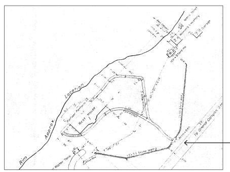
FIG. CD16: Site plan of the Hermit's Rest showing the original approach. Note location of corbel arch before relocation at arrow. Full drawing is contained in Appendix B, October 1934 (Kansas State Historical Society, Santa Fe Collection).
