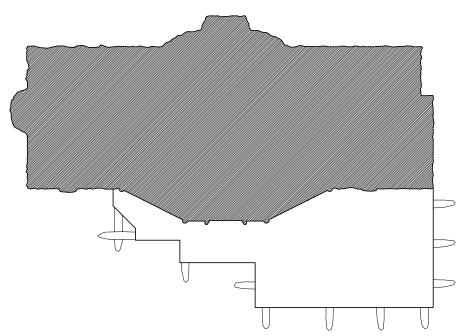
FIG. AT1: Option A for Porch Restoration. The west porch addition would be removed and the historic porch restored.
