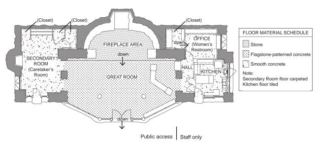
FIG. INT1: Floor Plan. Historic uses in parenthesis, 2007.
