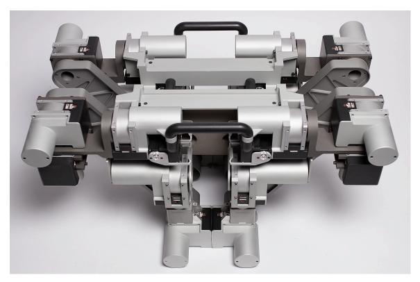
Above: OSCR-5 (On-Site Construction Robot) is a fully functional, automated hod-carrier built from scratch using custom designed servo motors, machined aluminum and 3d printed titanium parts. (The project was made possible by funding from the National Science Foundation and Autodesk, Inc.)
