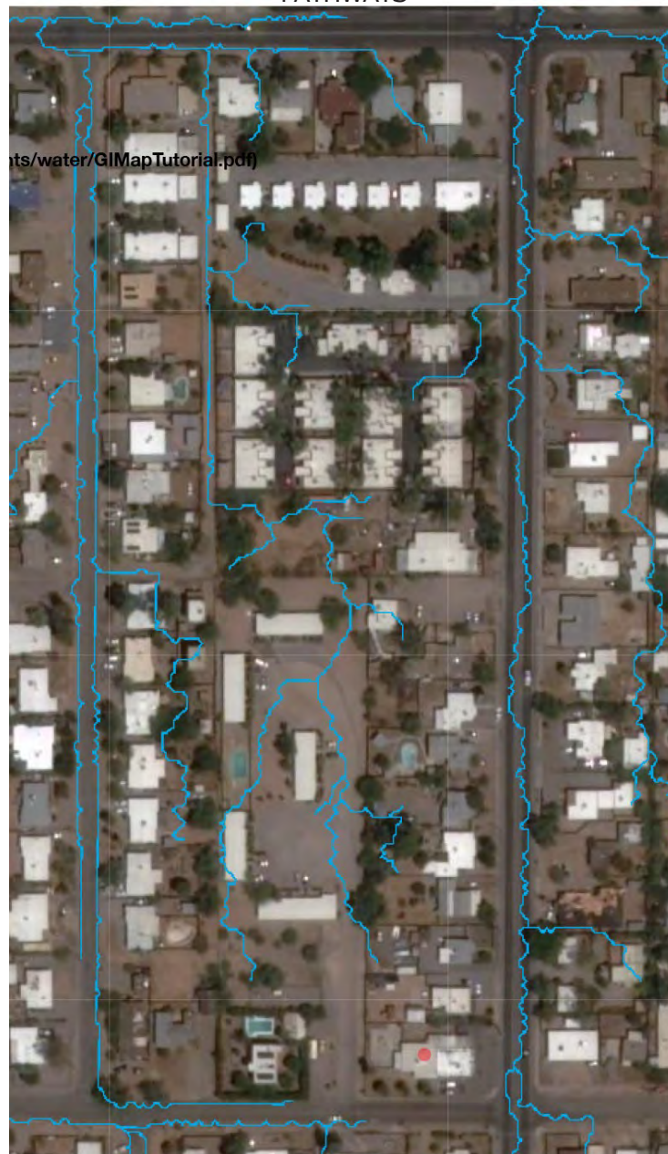
2008 IMPAIRED DRAINAGE PATHWAYS
