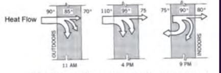
As daylight penetrates the tanks, the thermal mass is "charged", and can be directed into the house over an extended period of time.
