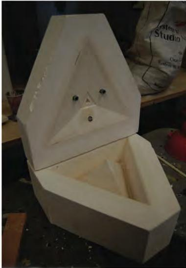
45. Pottery plaster molds for slip casting
