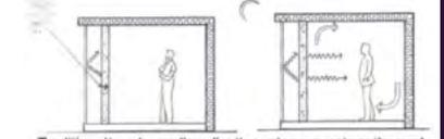
Traditional trombe-wall application using concrete as thermal mass. Water has nearly three times the heat capacity of concrete and can also serve as a day lighting source
