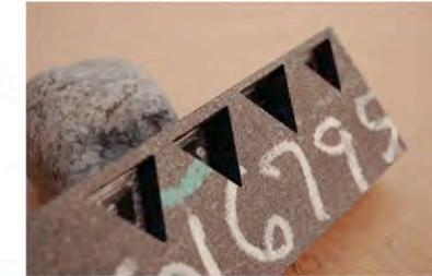
8. Machined graphite mold block
