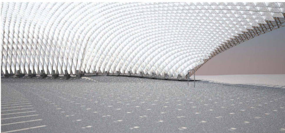
Simulated lighting condition using a high reflective ceramic. Reflectance(0) = 243,243,243 Reflectance(90) = 163,163,163 ND Scale = 1 Roughness = 95,55,0
