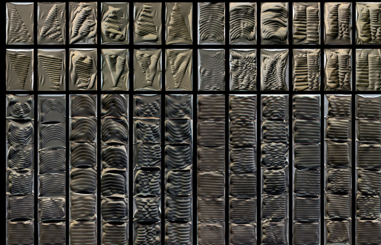
Laminated strip study set for finding the relationship between laminated pattern and resultant deformation
